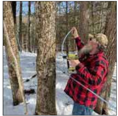
Running a new dropline from the tree to a mainline. Photo courtesy Goosebrook Meadows Sugar House
